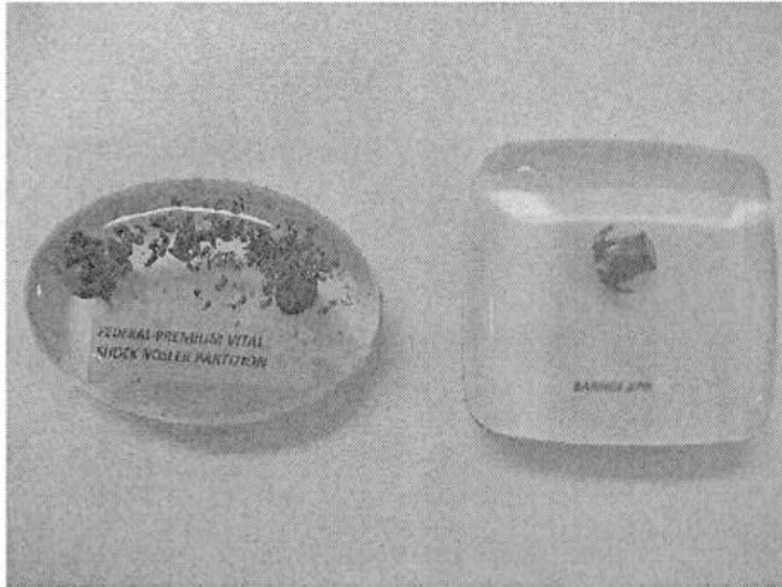
Figure 6: Lead (left) versus non-lead (right) ammunition after mass retention testing conducted by the Yurok Tribe.
