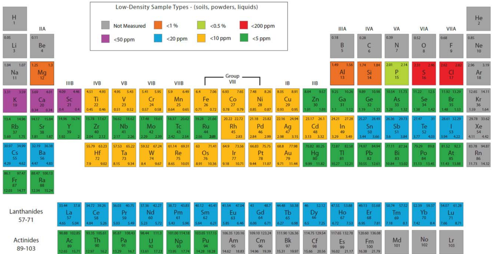
Fig. 3. Generalized limits of detection for the Delta PXRf by Olympus.
