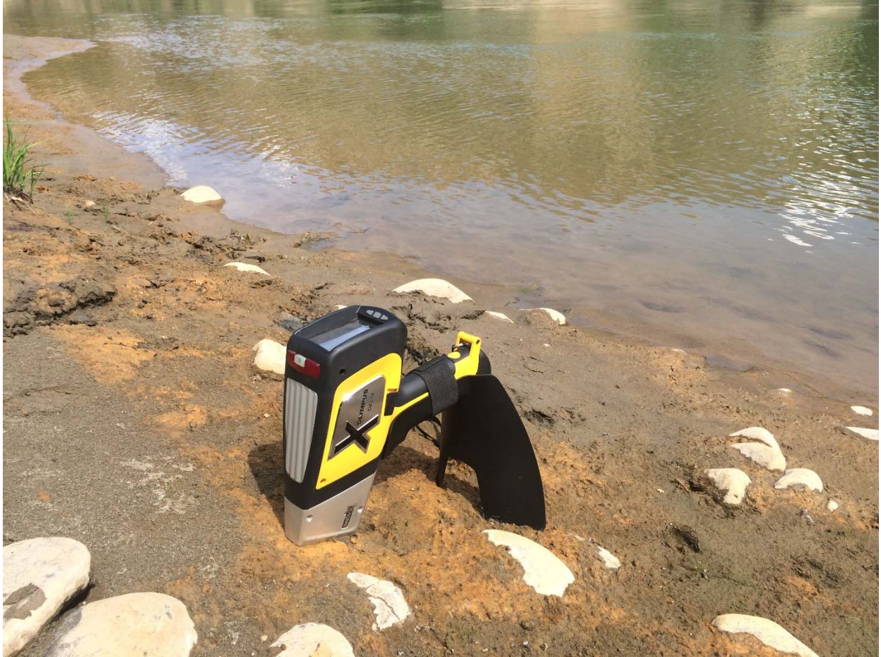
Fig. 4. Assessment of sludge laden sediment with portable x-ray fluorescence spectrometry along the banks of the Animas River in New Mexico.
